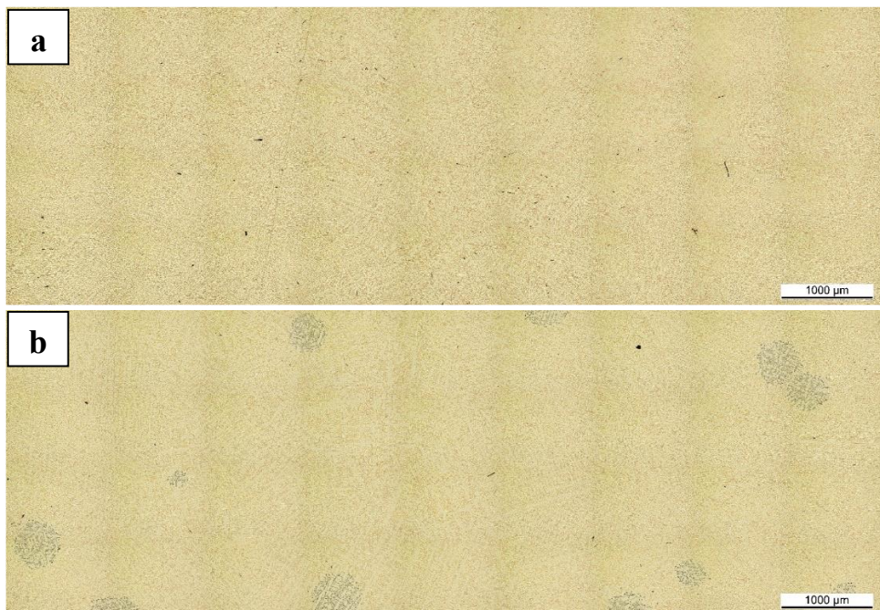
Figure 7.12. Graphite cluster in LS-CI after chill casting at (a) 1300°C and (b) 1400°C with a three-minute holding procedure.
