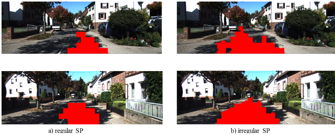
Figure 3.12: Road segmentation prediction with SP-CNN for two samples based on: a) fixed-size superpixels (Patches), b) irregular superpixels
