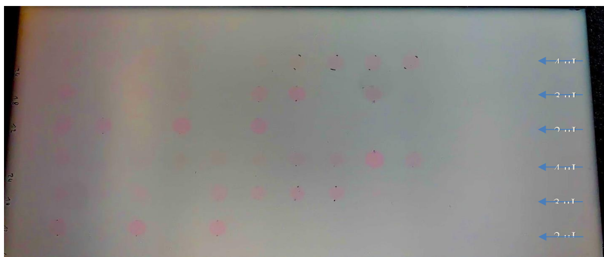
Figure 6-10: TLC plate where fractionation volumes of 2, 3 and 4 \mu\text{L} have been applied. Fractionation parameters: 10 \mu\text{L}/\text{min} flow rate, 0.1 mg/mL Rhodamine B solution, six longitudinal rows with 15 spots in one row.
