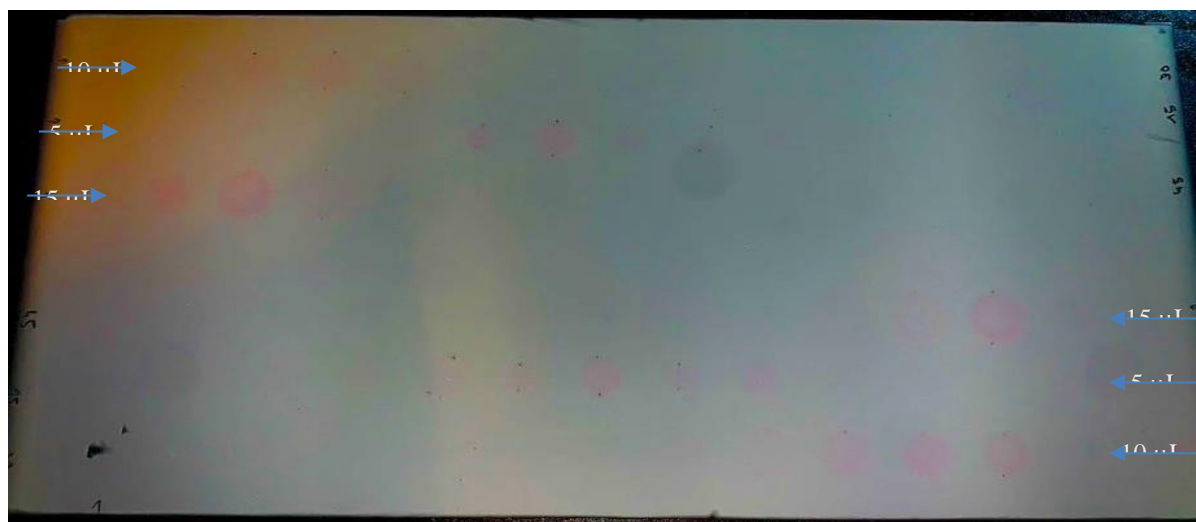
Figure 6-8: TLC plate where fractionation volumes of 5, 10 and 15 \mu\text{L} have been applied. Fractionation parameters: 20 \mu\text{L}/\text{min} flow rate, 0.1 mg/mL Rhodamine B solution, six longitudinal rows with 15 spots in one row.
