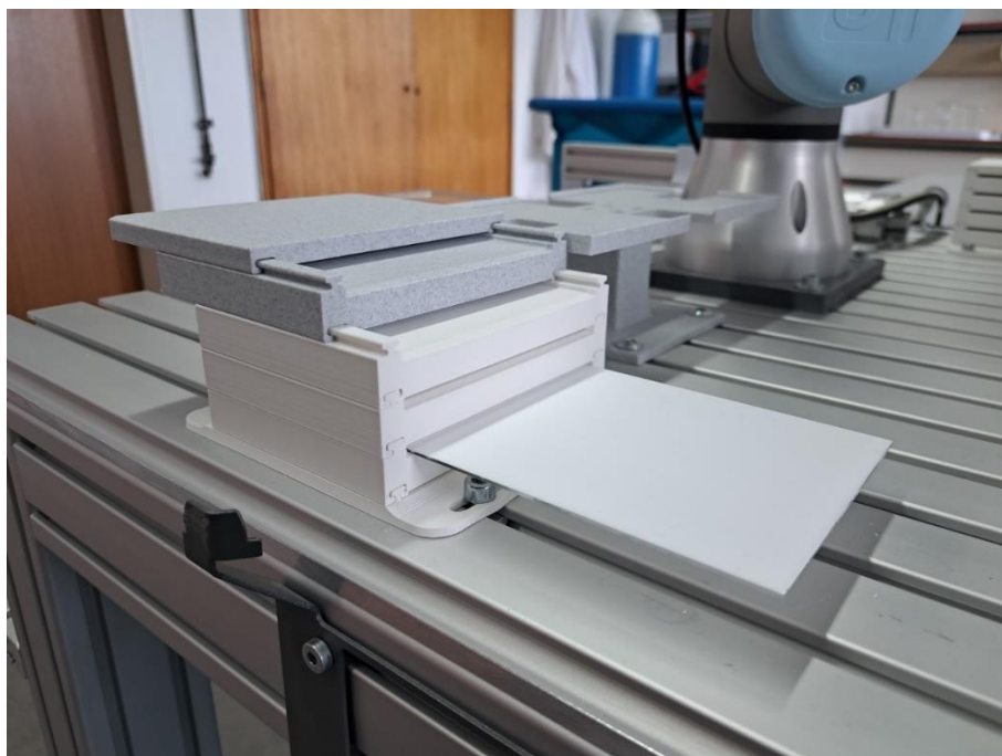
Figure 8-10: Photo of the modular plate storage system. The compartments and the lid are pushed onto the base using a guide rail. The plate with the sample is inserted into the holder.
