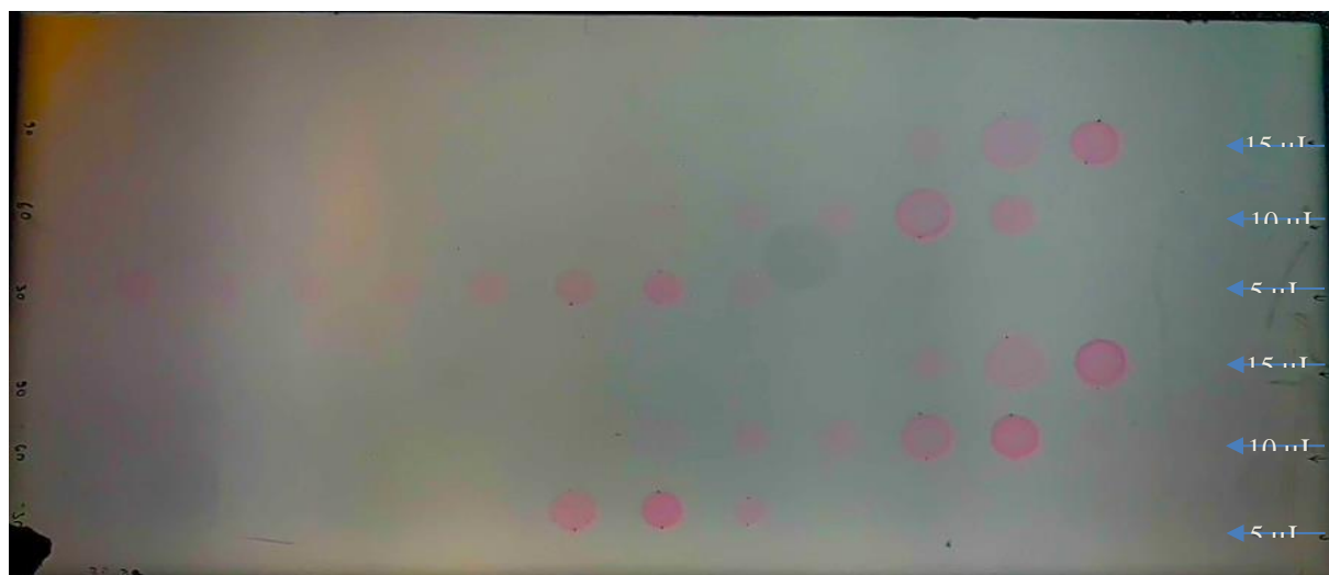
Figure 6-9: TLC plate with where fractionation volumes of 5, 10 and 15 \mu\text{L} have been applied. Fractionation parameters: 10 \mu\text{L}/\text{min} flow rate, 0.1 mg/mL Rhodamine B solution, six longitudinal rows with 15 spots in one row.
