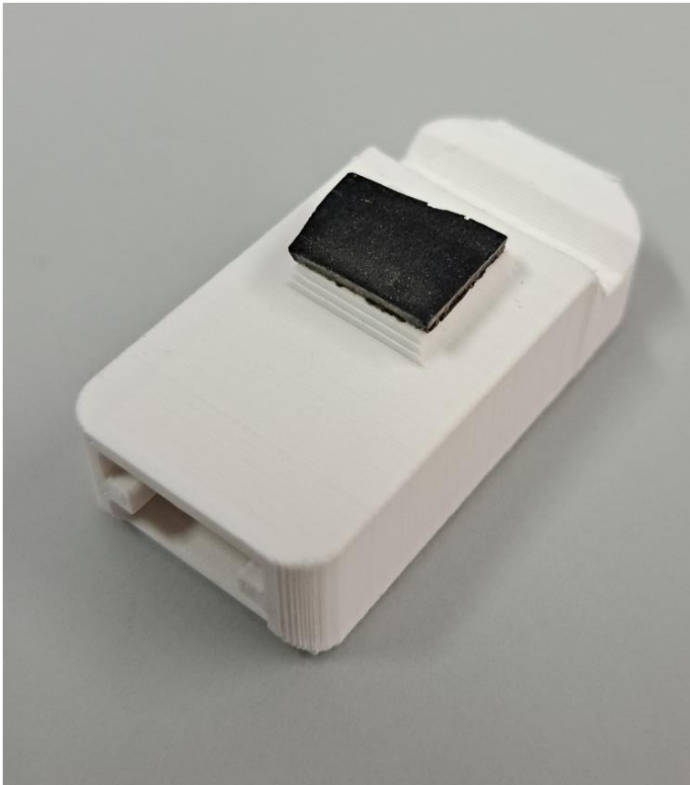
Figure 8-18: Gripper jaws for sliding onto the fingers of the gripper through the opening at the bottom. The elevation with the black anti-slip foil is used to grip the HPTLC plate from the side. The notch is for gripping from above.
