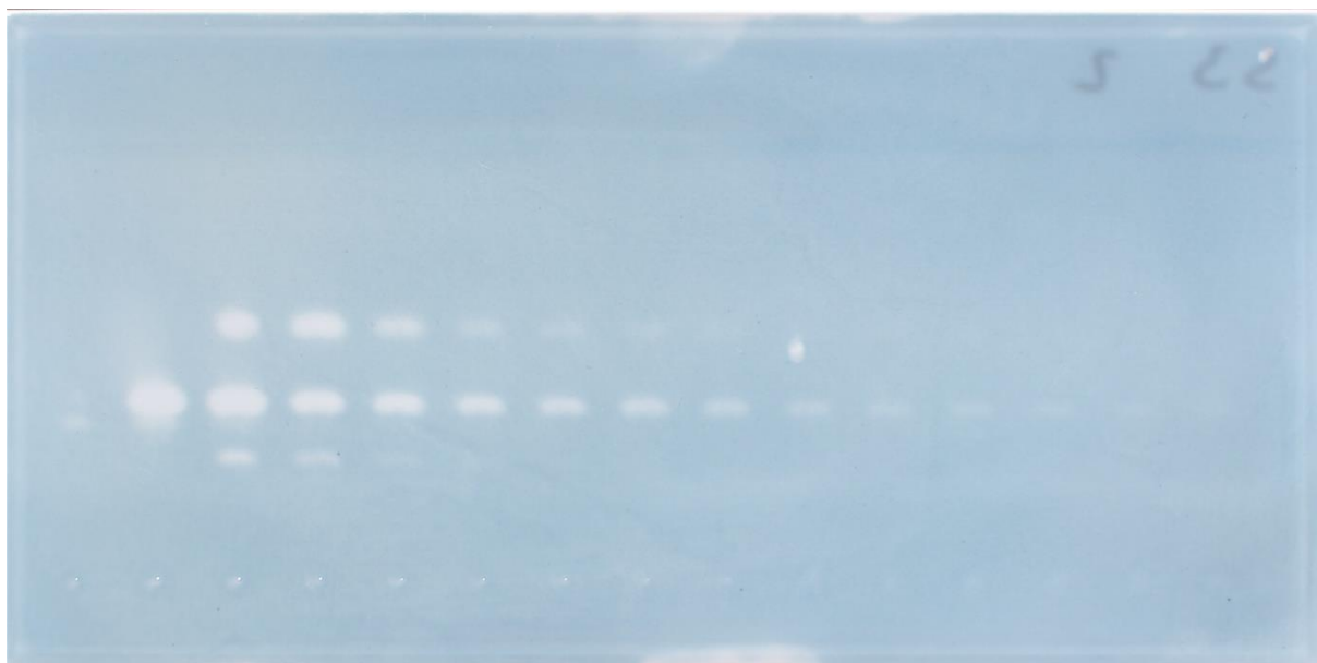
Figure 6-14: Image of the fractionated spiked water sample with malathion, chlorfenvinphos and parathion (from top to bottom row).
