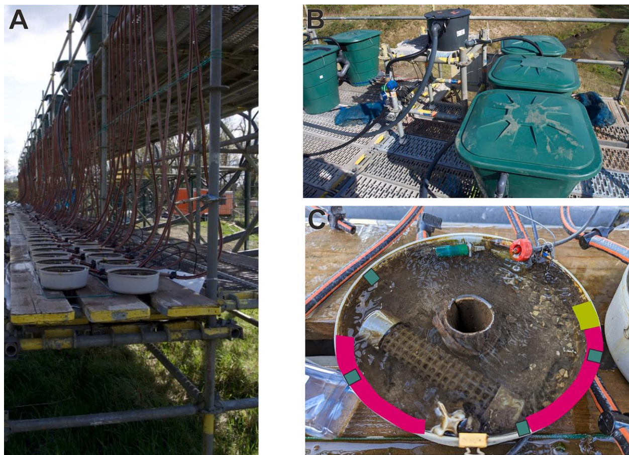
Fig. 1. ExStream experimental setup show A) circular mesocosms; B) header tanks (green) and small heating bucket (black); C) Inside the circular mesocosm channel showing the dripping line for salt treatment, the area scraped for biofilm recovery in light green, area scraped for different biofilm samples analysed in this study red, and areas where MINI-PAM II measurement were done (dark green).
