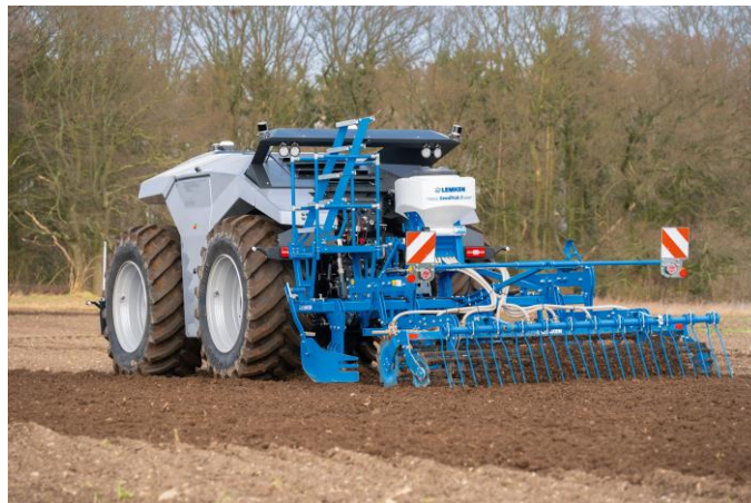
Figure 1: Combined Powers machine [1] – combination of a smart implement with an autonomous towing vehicle (image source: LEMKEN GmbH & Co. KG)
