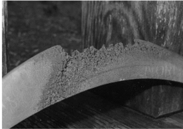
Fig. 3 End stage of cavitation erosion of a ship propeller (adapted from [15]).
