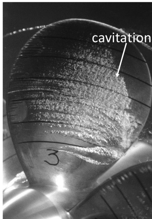
Fig. 2 Cavitation occurring near a ship propeller (adapted from [15]).
