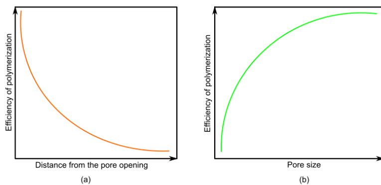
Figure 4.98. (a) Efficiency of polymerization decreases as the distance from the pore opening increases into the pore, and (b) Efficiency of polymerization increases with increasing pore size
