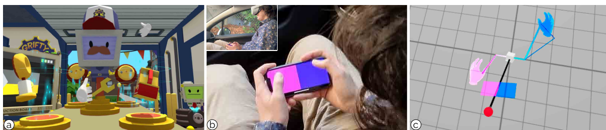
Figure 6.1: HandyCast is a scene-agnostic input technique for bimanual and full-range control in expansive virtual environments under physical space constraints, using touch and motion of a hand-held smartphone. HandyCast enables users to (a) operate rich Virtual Reality environments as in Job Simulator with two virtual hands (b) by sensing embodied interaction from as little physical space as a car’s passenger seat as users move, turn, and touch the phone like a controller from the comfort of their lap. (c) HandyCast implements a pose-and-touch transfer function that individually fuses and amplifies phone and touch motions into position, rotation, and selection parameters for either virtual hand. Building on visual-inertial odometry to retrieve the 6D phone pose, HandyCast brings the 3D input control common in stationary setups with two hand-held controllers to mobile settings , using just a headset and a smartphone anywhere without the need for external tracking.
