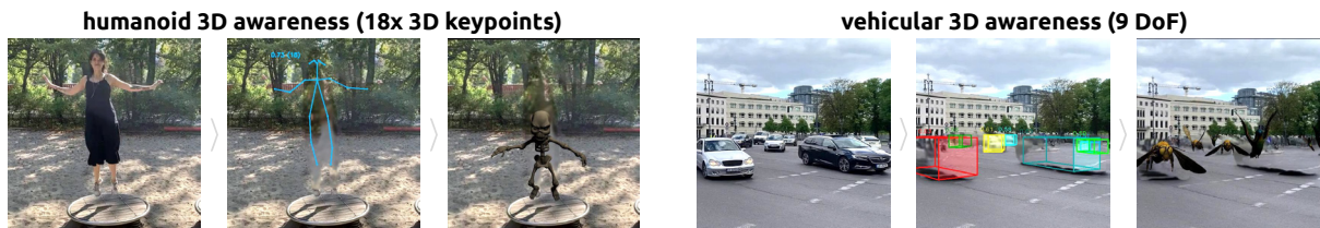
Figure 4.4: Examples for our 3D-pose-aware object substitution approach. 3D pose estimation is performed for vehicles (top) and humans (bottom). Vehicles poses are estimated as oriented 3D bounding boxes. Human poses are estimated as 3D joint keypoints.
