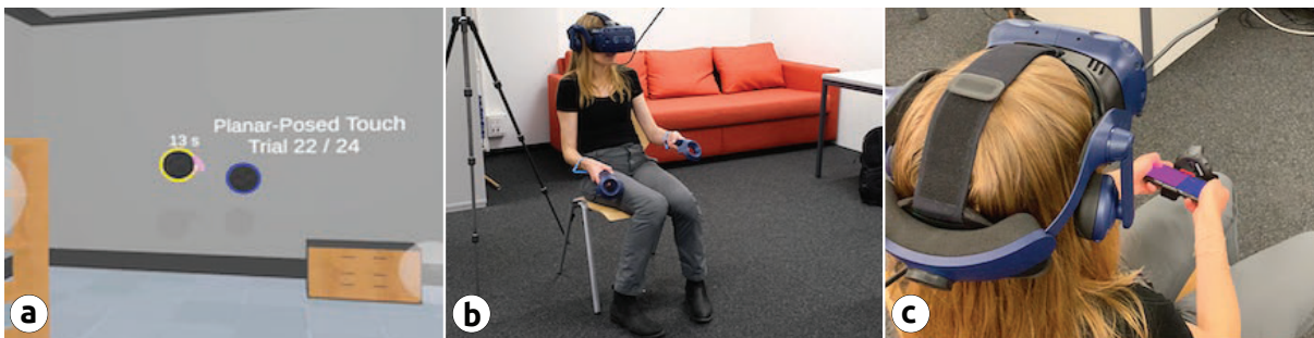
Figure 6.6: Apparatus for our full-range study. a) Our Unity app rendered the study environment, displayed through a VIVE Pro Eye. b) For Go-Go input, participants used the VIVE controllers. c) For all phone techniques, a VIVE tracker provided the pose of an iPhone 11 Pro, which relayed touches to Unity.
