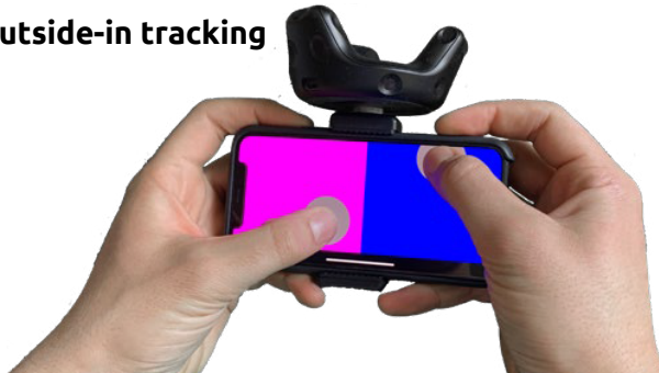
Figure 6.5: Users hold the HandyCast input phone like a gamepad, with each thumb operating in a single touch zone. For usage in common VR games, HandyCast can use inside-out tracking with no additional tracking hardware needed. For our two evaluations, a VIVE tracker is mounted to the phone allowing us to separately investigate interaction performance and tracking effects.
