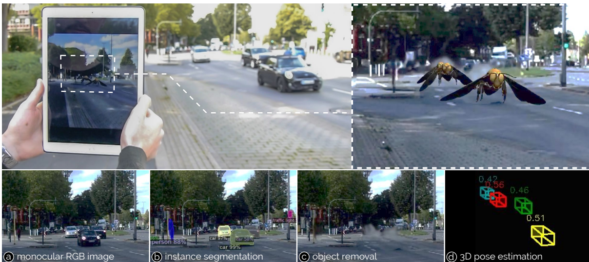
Figure 4.1: TransforMR is a video see-through mixed reality system for handheld devices that performs 3D pose-aware object substitution to create meaningful mixed reality scenes, enabling applications such as alternate mixed realities or real-time virtual character animation in context. (a) From just the monocular color camera of a mobile device, (b) TransforMR performs instance segmentation, (c) object removal, and (d) 3D pose estimation to substitute objects with pose awareness (top right).
