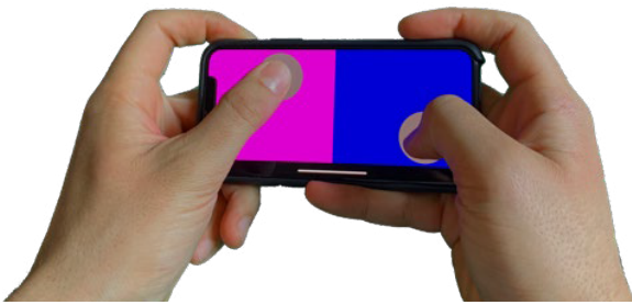
Figure 6.5: Users hold the HandyCast input phone like a gamepad, with each thumb operating in a single touch zone. For usage in common VR games, HandyCast can use inside-out tracking with no additional tracking hardware needed. For our two evaluations, a VIVE tracker is mounted to the phone allowing us to separately investigate interaction performance and tracking effects.
