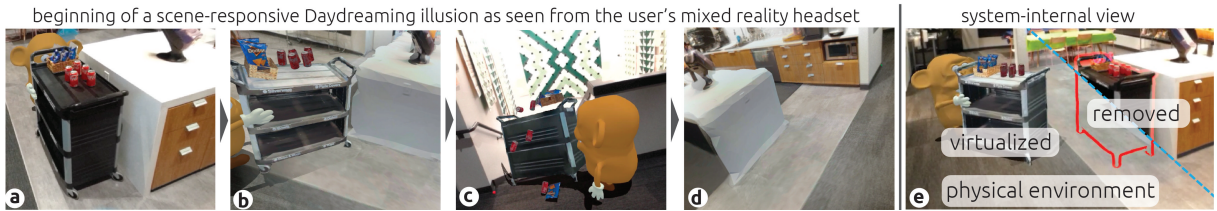
Figure 5.1: We present Scene Responsiveness, the visual illusion that virtual actions affect the physical scene. ① Wearing a video-passthrough Mixed Reality (MR) headset, a user sees an authentic video view of their physical environment, captured with the externally-facing headset cameras. A virtual monkey character is situated and coherently occluded in the otherwise unmodified physical space, grabbing the PHYSICAL cart. ② As the monkey starts dragging the cart, the object toggles its reality state to VIRTUALIZED just-in-time. Just-in-time virtualization is coherence-preserving , so the cart still throws its shadow onto the physical scene and the now seemingly empty surface. ③ To the user, it appears as if the monkey drags the physical cart and throws it down the staircase. Virtual shadows and collisions render coherently. ④ It appears as if the physical cart is gone. ⑤ Of course, what the user sees is just an illusion. The physical object did not move but was just masked from the user’s view, blending seamlessly with the video passthrough. Everything seen in the debug capture, incl. the red object guardian outline and the revelation lens in the top-right corner is part of the system debug view. The figure gives an authentic impression of the visual fidelity in the headset. However, please watch the accompanying video for a full impression of the visual experience.
