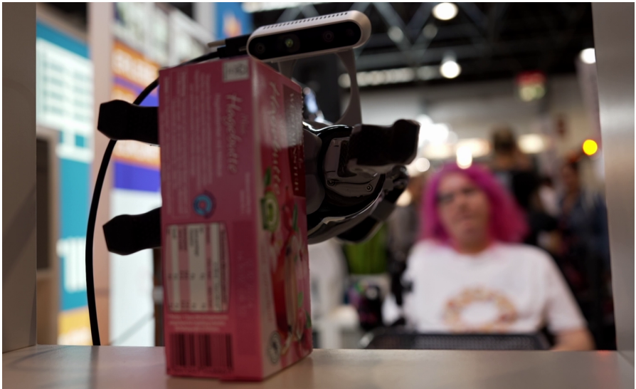
Figure 5.1: Grasping an object from a shelf by using ADMC. The interaction and feedback methods for our AI-enhanced assistive robot were evaluated with the target group. Participants were tasked with picking up various objects from a shelf and placing them into a basket on a table in front of them. The ADMC approach was assessed using three different input devices: head-based controls, assistive buttons, and a joystick. © Matthias Kraus, masapido Filmproduktion
