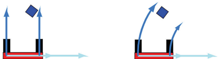
Figure 2. The simulated robot with two out of the four cardinal DoFs (left) and two adaptive DoFs (right) [6].
