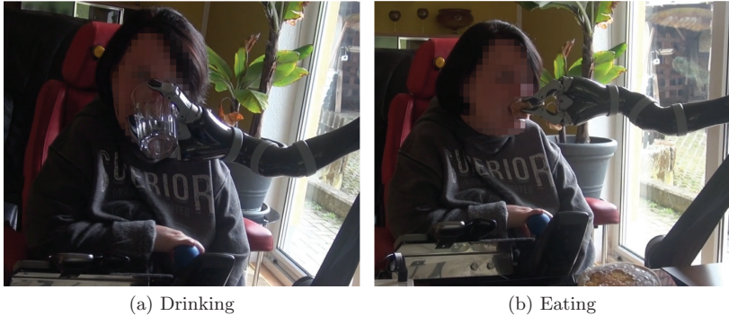
Fig. 5. Observation on the use of a robotic arm (JACO) for the consumption of food and drinks
