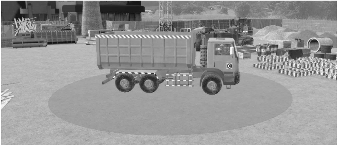
Figure 5.8: Single detection zone around a vehicle
