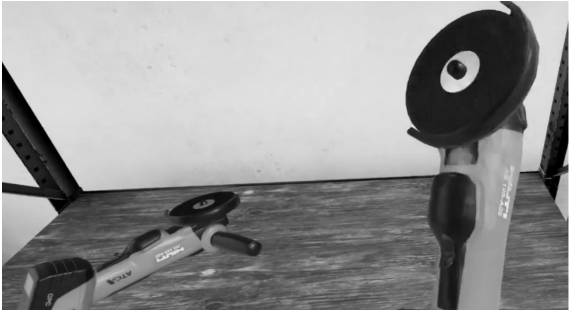
Figure 6.1: An angle grinder with handle (on the left) and an unsafe one without handle (right).
