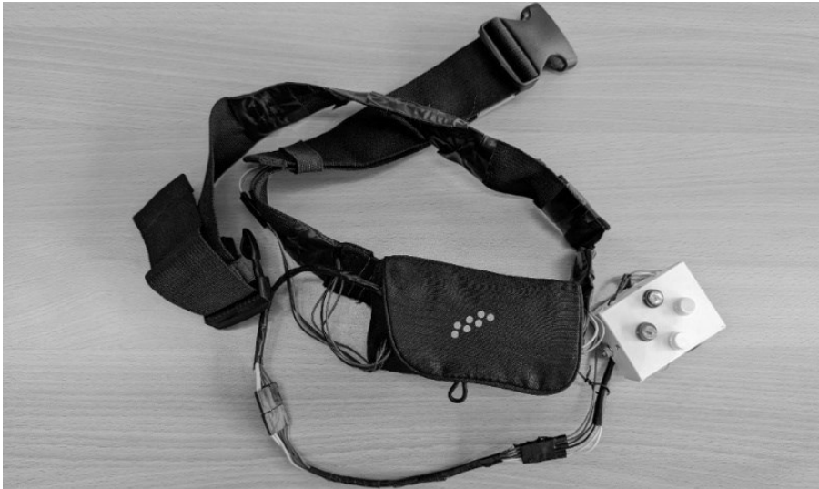
Figure 4.2: Abdominal (waist) belt with vibration motors and the input control
