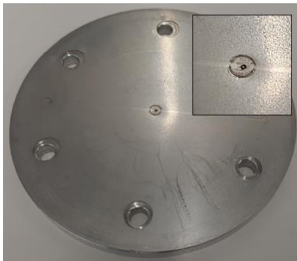
Figure 35: Surface suffering from metal-on-metal interactions of the mesh plate with 0.05 \mu\text{m} holes after several weeks of use.
