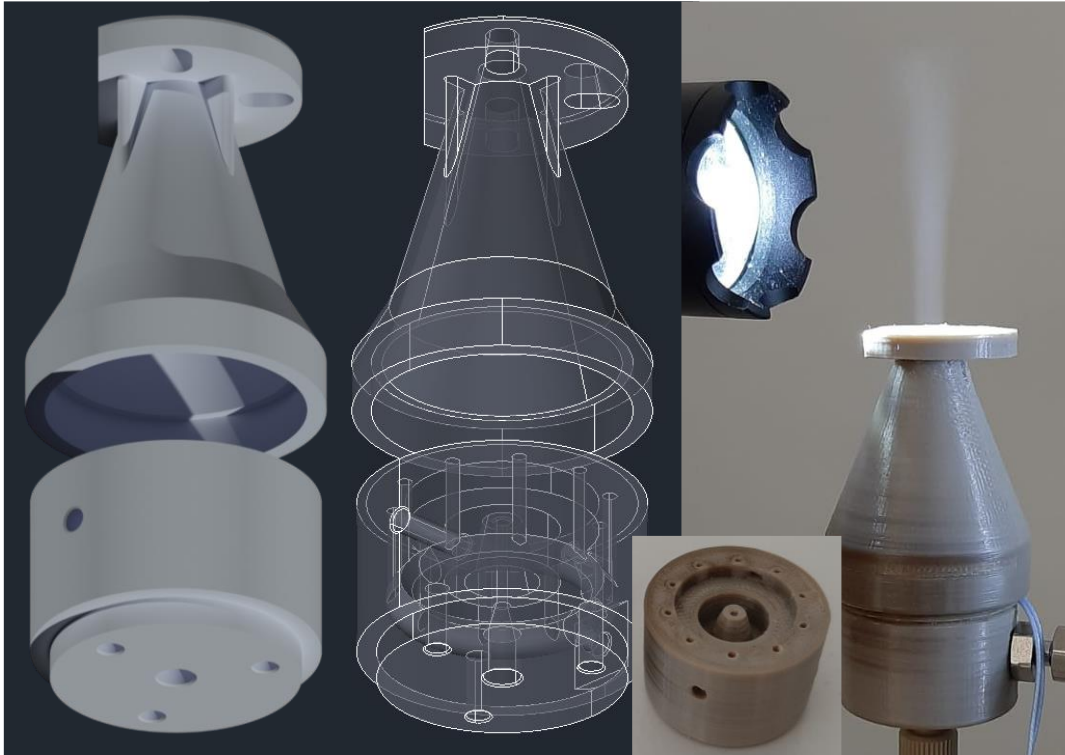
Figure 72: Focusing cone for the sprayed liquid in rendered view (left), X-ray view (middle), and operating with a flowing liquid supply and auxiliary nitrogen gas (entry at the side).
