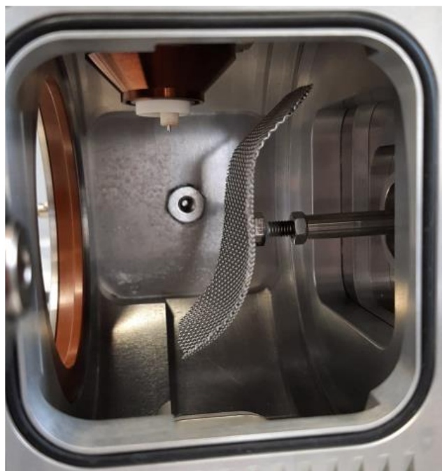
Figure 39: Repeller 7, a three-dimensional steel mesh formed in armchair-formation.
