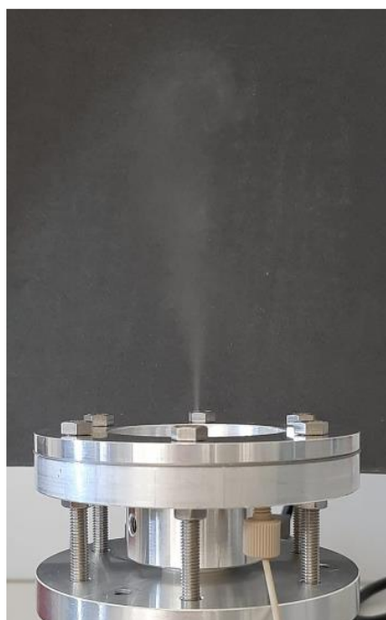
Figure 23: Operating Hitachi nebulizer: 300 \mu\text{L min}^{-1} methanol was supplied through the PEEK capillary and the piezo-element was operated at 4 W.
