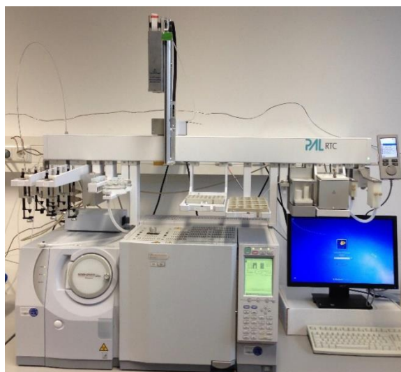
Fig. S 6.4. Picture of the set-up used, including PAL RTC head, rail and controller, GC-MS QP2010 Ultra and computer. The PAL modules used in this study (from left to right) were: two parking stations, SPME Fiber Conditioning station; small and big washing stations, two tray holders, vortex mixer and agitator.
