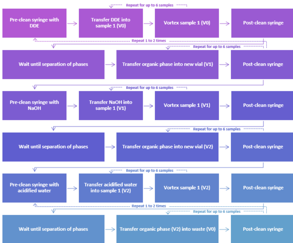
Fig. 6.3. Simplified overview of the liquid-liquid extraction steps. Several vials are needed for the same sample, denoted as (Vn). Optional steps denoted with dotted lines.
