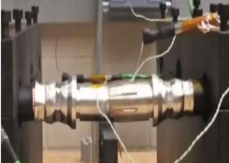
Fig. 3.9: Connector joule heating measurement setup
