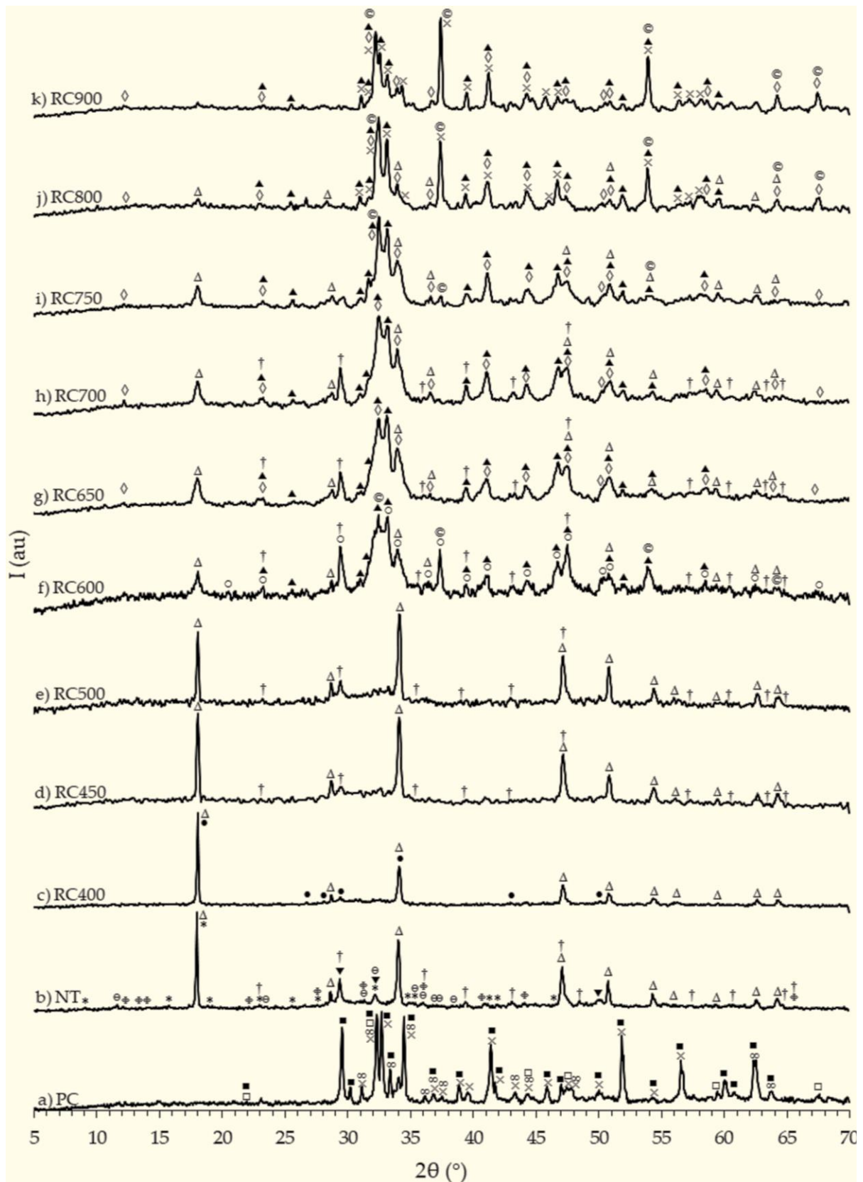
Figure 2-21: XRD analysis of PC, NT and RC. \Delta portlandite; \dagger calcite; * ettringite; \infty gypsum; \copyright CaO; \blacksquare C_3S ; \bullet tobermorite; \blacktriangledown C-S-H; \times \beta - C_2S ; \blacktriangle \alpha' - L - C_2S ; \circ C_3A ; \square calcium aluminum iron oxide; \diamond brownmillerite; \phi alumhydrocalcite; \oplus calcium aluminum oxide carbonate hydrate [167].
