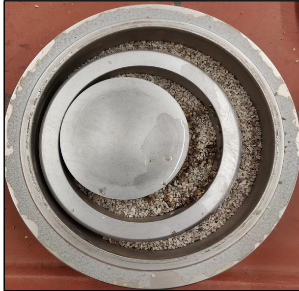
Figure 3-5: The filled grinding jar during the milling process.
