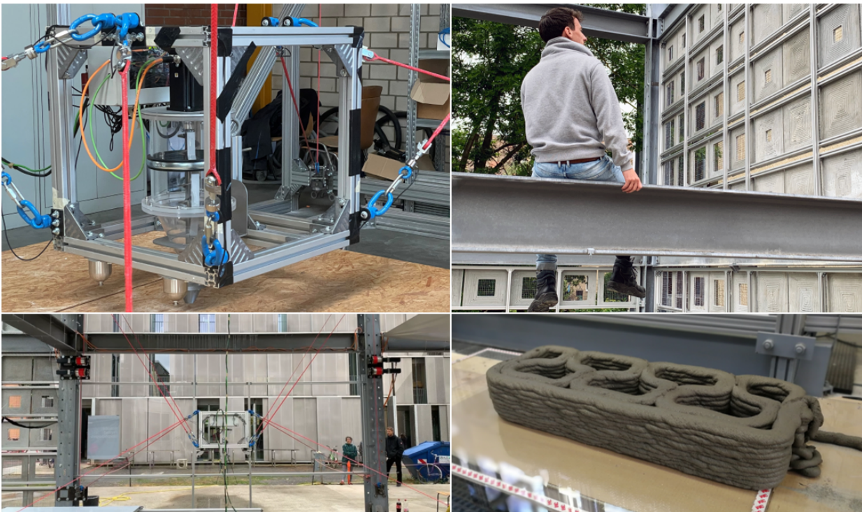
Figure 6.2: A CDPR for concrete 3D-printing, facade elements installation and test specimen.
