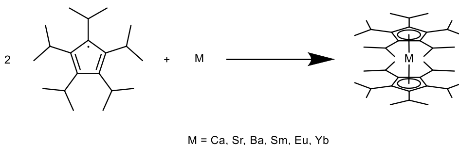
Scheme 18: Synthesis of decaisopropyl metallocenes by reaction of decaisopropylcyclopentadienyl radical with different metals. [122,123]
