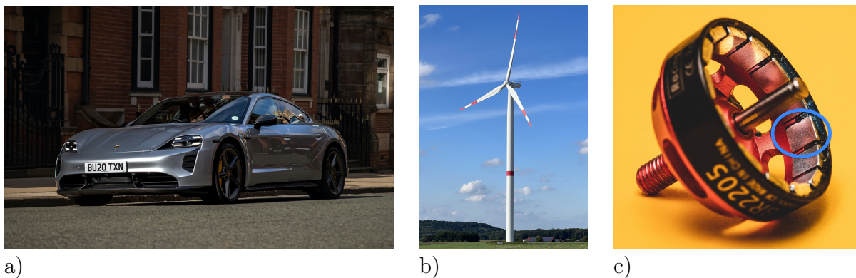
Figure 1.1: Strong and efficient permanent magnets can be used to enhance a) the electric transportation (KEMP [2021]) and b) the energy conversion (VORWERK [2023]), since they are c) important components of electric motors (one magnet highlighted in blue circle) (BAUMEISTER [2020]).
