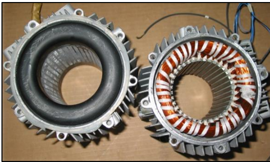
Figure 1.18 – Potted windings (left) vs non-potted windings (right) ( Dreisilker 2023 ).
