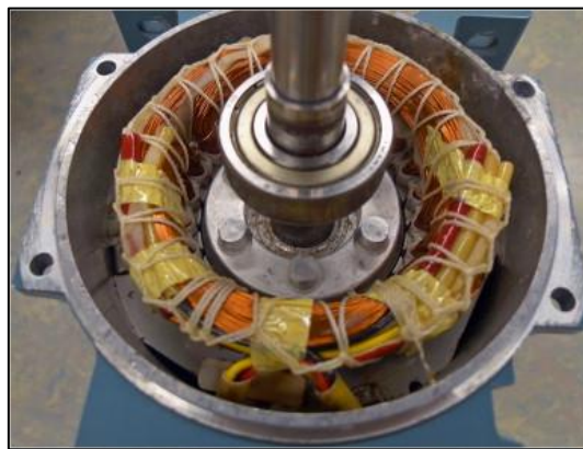
Figure 1.16 – Final aspect of the end-windings with all the insulation layers (Hultman and Leijon, 2013).
