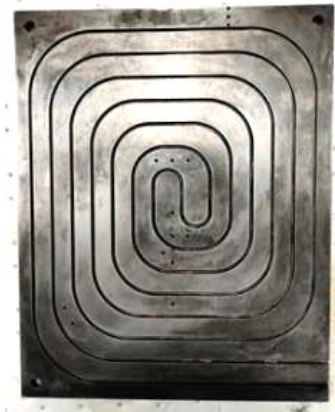
Figure 2.5 – Upper surface of the heater. The electrical resistance is installed inside the carved canal.
