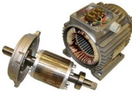
Figure 1.6 – Example of an induction motor with a squirrel cage rotor ( Wikipedia 2023a).
