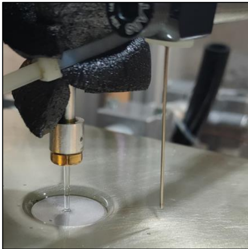
Figure 2.15 – Thermocouple for measuring the temperature of the liquid film along the plate-normal direction.
