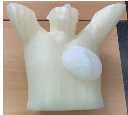
Fig. 1: Hydrogel breast phantom prototype with 2x2-hour-FTCs. Fig. 2: Silicone breast phantom with the infill 94A: 6B
