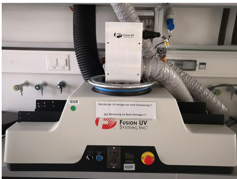
Figure 3. Image of the alignment of mercury conveyor from Heraeus with integrated microwave lamp.
