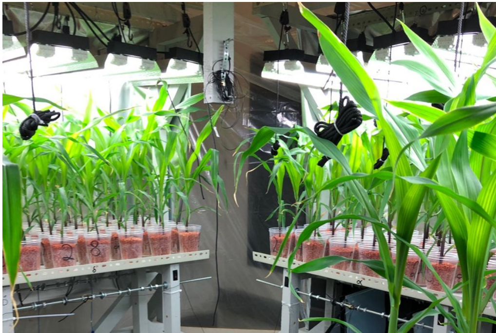
Figure 3.1: Indoor greenhouse test rig with potted maize plants equipped with artificial lighting, Chair SRS, University of Duisburg-Essen, Germany.
