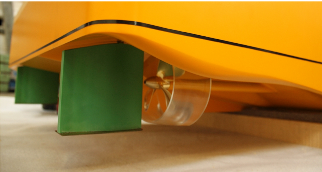
Figure 4.5: Detailed side view of the propulsive and steering devices arrangement.
