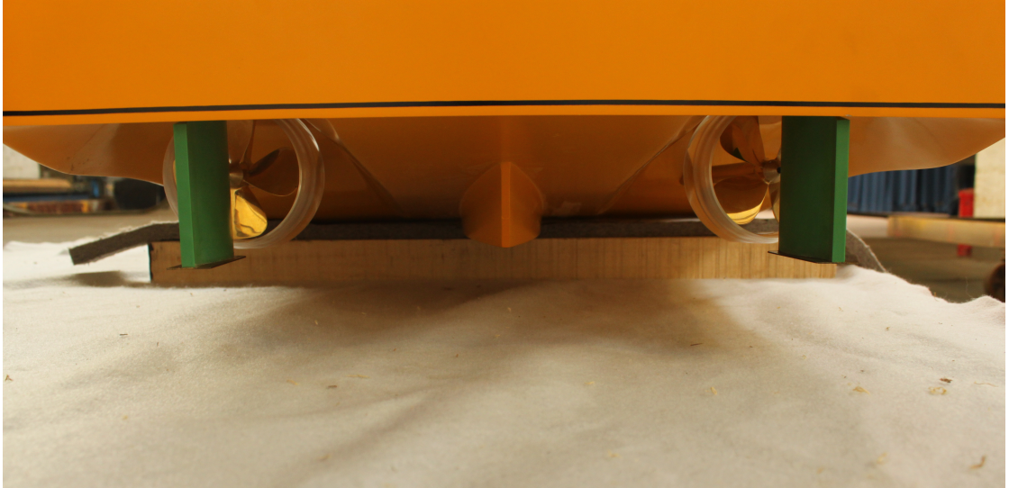
Figure 4.6: Detailed stern view of the propulsive and steering devices arranged in the tunnels of the pusher-boat.
