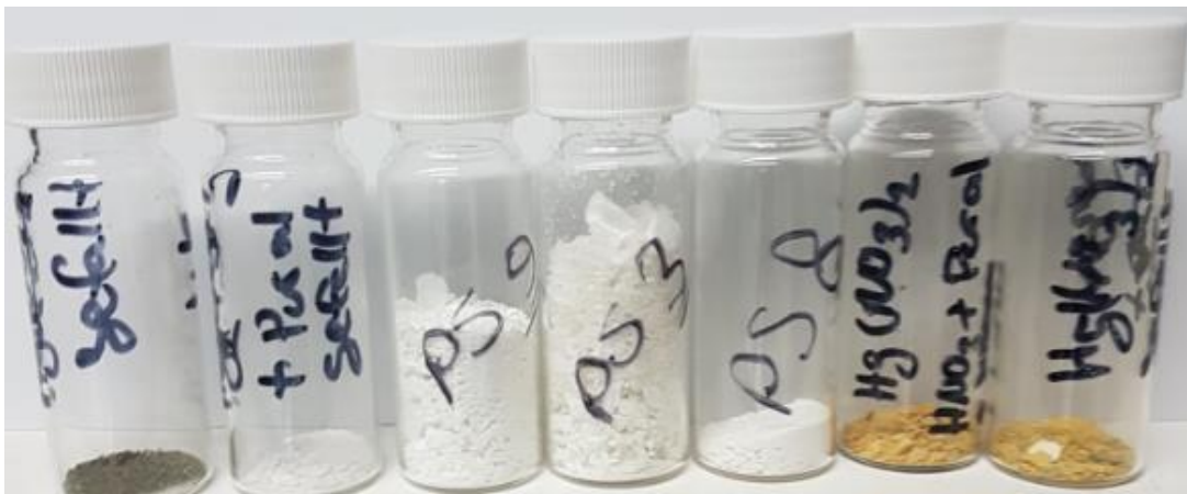
Figure 53 Picture of the different precipitated samples, from left to right: \text{Hg}_2(\text{NO}_3)_2 (black); \text{Hg}_2(\text{NO}_3)_{2,\text{aq}} (grey); \text{Hg}(\text{NO}_3)_{2,\text{aq}} (white); \text{Hg}(\text{NO}_3)_2 (yellow)
