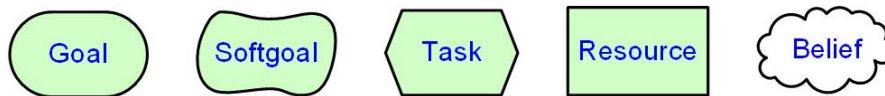
Figure 2.3: i^* notation for the intentional elements goal, soft goal, task, resource, and belief.
