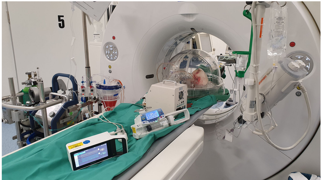
Fig. 2 Actual setup. The lower lung lobe is positioned in the computed tomography gantry
