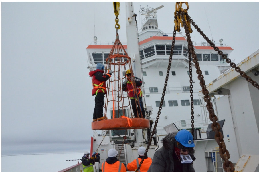
Figure 42 Two persons are lifted onto the ice for sea ice coring with help of the basket.
