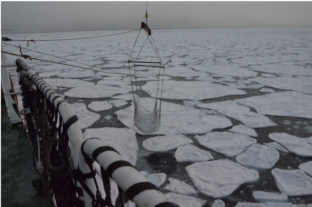
Figure 38 A pancake ice floe for testing is lifted out of the water.
