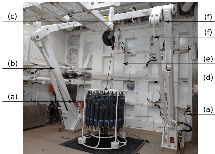
Figure A 4 A-frame (height 4.79 m, the arm is 2.00 m long) of the SA Agulhas II. The door (e) is opened automatically, the A-frame can be swung out (b), the frazil sampler is attached to the small roll (c), loops for the opening and closing ropes of the frazil ice collector (f), operators can stand on the sides of the frame (a) to hold the sampler into position.
