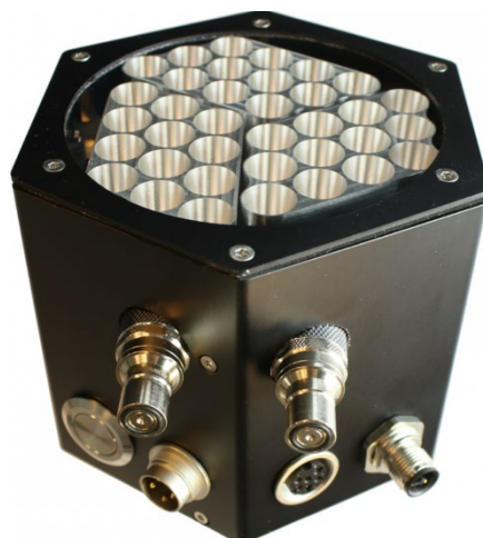
Figure 4.4. Image of the LED array (OLM-046A-c, made by OSA Opto Light), at 268 nm CWL with 15 nm FWHM of 15 nm, used as a source of UV illumination.
