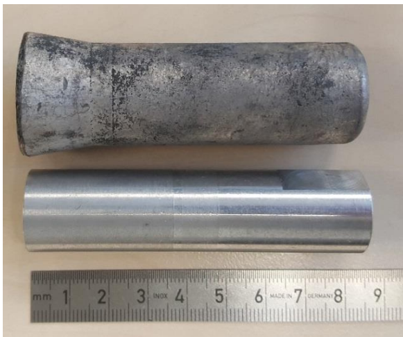
Figure 10: Cast rods & machined consumable studs.
