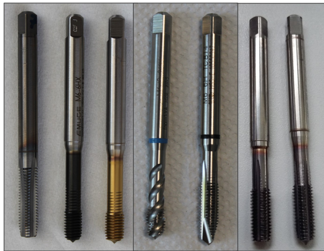
Figure 2.11: Various tools for cut or form tapping
