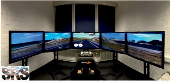
FIGURE 5. Driving simulator, chair of dynamics and control (SRS, Uni-DuE).
