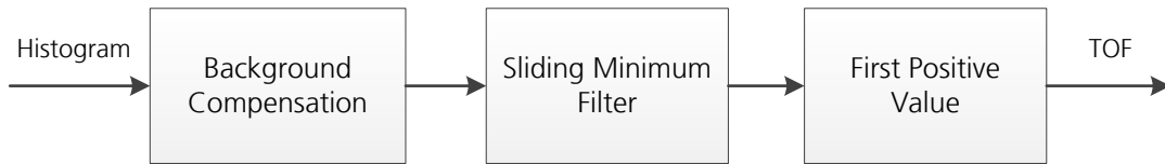
Figure 5.4: Sequence diagram of the minimum filter routine.
