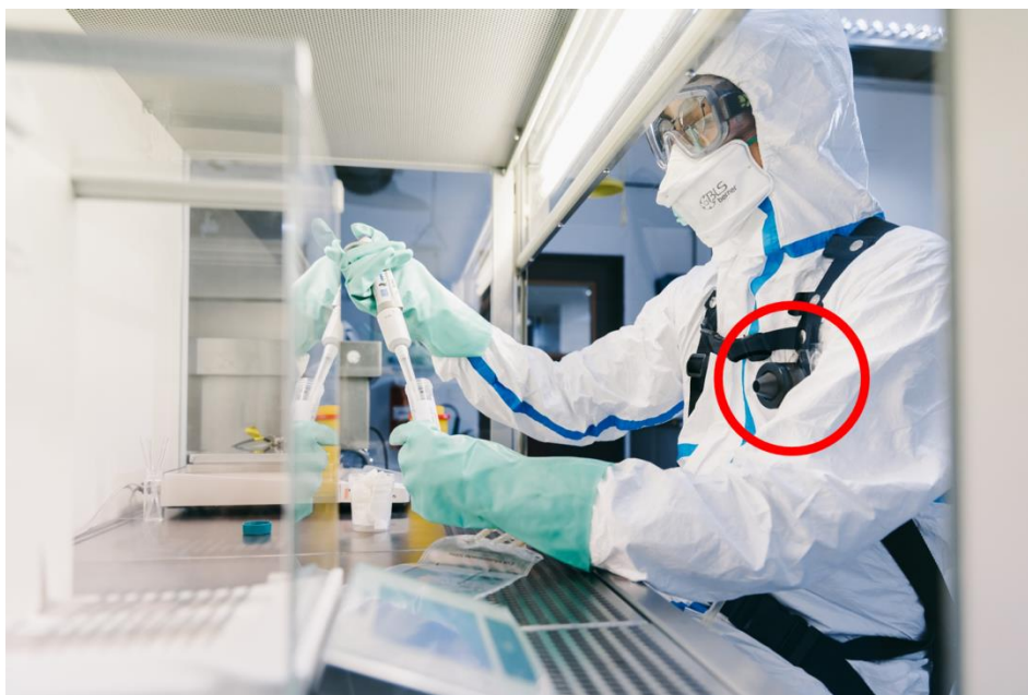
Figure 7-11: Depiction of a person wearing the personal air-sampling pump. The sampling head is highlighted by a red circle.
