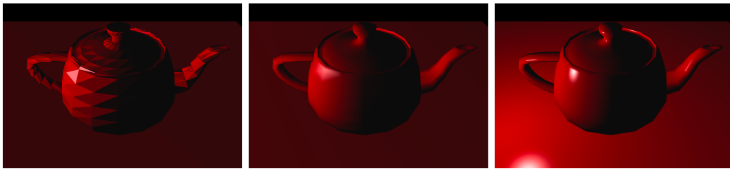
Fig. 2.1 The famous Utah Teapot by Martin Newell [288] lid with three different lighting models. Left: Flat Shading (single color per triangle) Middle: Gouraud Shading (per vertex lighting) Right: Phong Shading (per fragment lighting).
