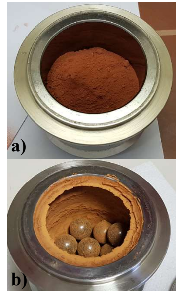
Figure 3.3 Change in color from reddish (a, after homogenization) to orange (b, after mechanochemical activation).
