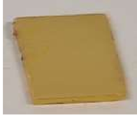
Figure 4.5 A PFN film deposited on STO (001) by PLD.
