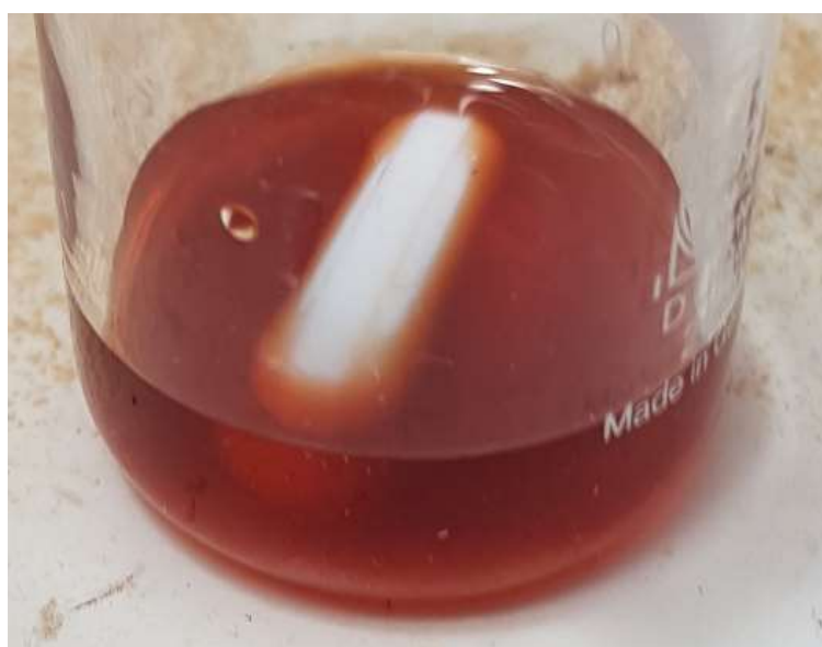
Figure 4.23 Sol gel solution after mixing precursors together.
