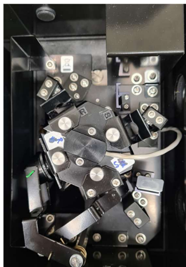
Figure 2.14 a) UV2600 integrating sphere attachment. b) Light path [141]
