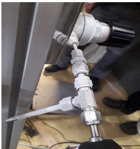
Figure 2: Freezing the single-valve sampling line during gas sampling.
