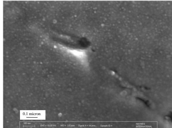
Figure 3. High magnification of mill annealed 282® alloy showing well dispersed very fine intragranular gamma prime particles. Particle sizes are typically less than 5 microns.
