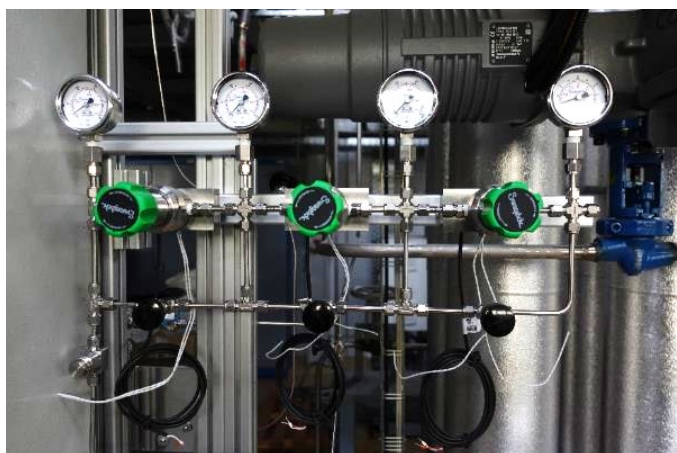
Figure 3: The three-stage sampling line employing gradual pressure reduction of the sCO 2 in the experimental loop.
