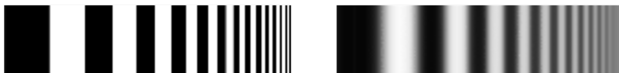
Figure 3.4: Comparison of optical performance of an ideal (left) and error-prone system (right) [95].
