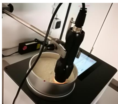
Fig 3.6 Photo of the experimental set-up of a flour measurement with the MicroNIR in combination with the IAS 3100 NIR spectrometer
