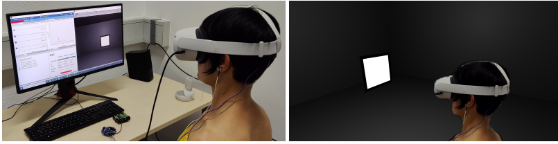
Figure 9.3: For our study apparatus, we use an Oculus Quest 2 VR-HMD and OpenBCI Ganglion EEG board. Left: A participant wearing a VR-HMD focusing on a stimulus. Right: The same participant in VR, focusing on a black and white flickering square.
