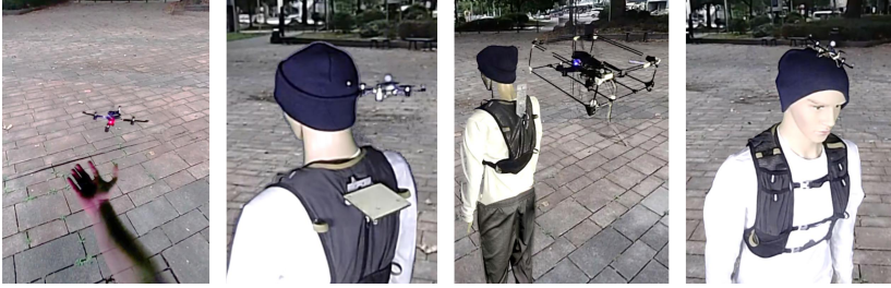
Figure 11.6: The human body allows for fast and autonomous take-off and landing of drones. We conducted an online survey and a follow-up study with 360° VR videos to investigate the landing suitability of various body locations (e.g., hand, back, or head).
