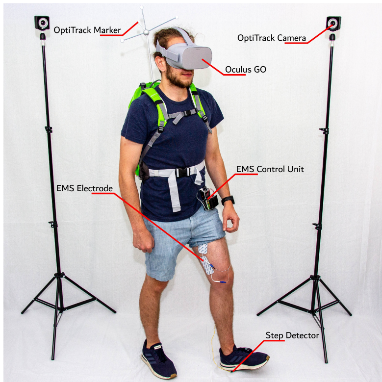
Figure 6.2: The Infinite Walking setup includes cameras and markers for optical tracking, an EMS Control Unit and Electrodes for actuating, a Step Detector for properly timed actuation, and an Oculus Go for displaying the VR scene (staged scene).
