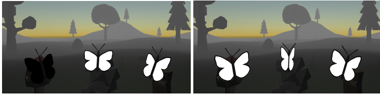
Figure 9.8: The VR mini-game we developed as a showcase for our investigated stimulus types . Left: stimulus with black and white flickering butterflies wings. Right: stimulus with butterflies flapping their wings. Both: from left to right, the butterflies were flickering or flapping with 6, 8, or 10 Hz.
