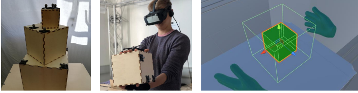
Figure 8.8: Left: We track haptic props to enhance the virtual experience. Middle: A VR user investigating a virtual box while holding a prop. Right: The virtual view. The haptic prop is rendered transparent (outer green box). To the user, only the solid green box was visible in virtual reality.
