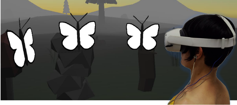
Figure 9.1: A VR user looking at butterflies. The butterflies elicit SSVEP responses through either flickering or flapping wings.
