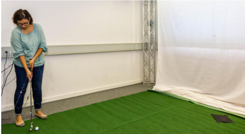
Figure 6.1: A user testing GeniePutt in a mini-golf scenario. The EMS system supports the user by turning the wrist so that the club faces the target.
