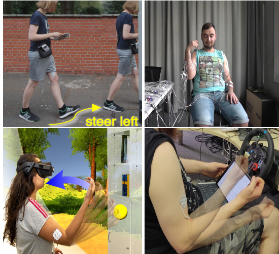
Figure 3.1: Examples of Electrical Muscle Stimulation for human actuation. The user’s leg is actuated to change the walking path [319] or the arm is actuated to communicate emotions [146], prevent hitting physical objects while in virtual reality [95], and to communicate take-over request in autonomous vehicles [97] (left to right).
