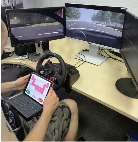
Figure 10.2: The final setup of the simulation used in the study. We presented the view on three displays (i.e., one for the front and two for the side), along with a Logitech G29 driving wheel. The non-driving task is displayed in a tablet placed on the driver's lap.
