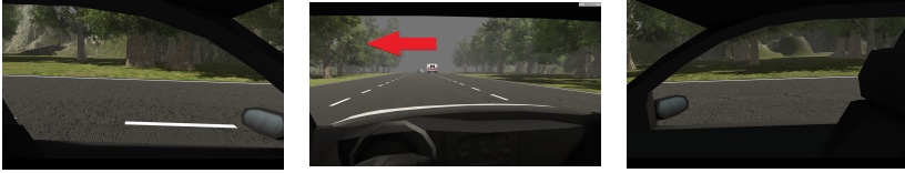
Figure 10.3: The autonomous vehicle driving on a 3-lane highway road, when it encounters an accident blocking the right and the middle lanes. A visual TOR is issued, indicating the free open lane for crossing.
