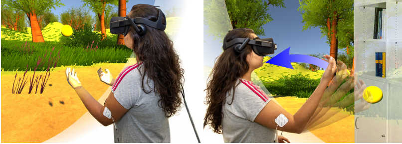
Figure 9.1: SaVR uses Electrical Muscle Stimulation (EMS) to prevent users from hitting physical obstacles while experiencing Virtual Reality (VR) applications. EMS actuates muscles resulting in an automated movement that pulls the arms away from a physical obstacle and thus increases the safety of the user.
