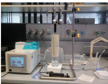
Figure 5.36 A photograph of the shaping equipment with a paper cylinder to protect the falling routes of microdroplets.
