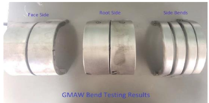
Figure 12. Photograph of bend test specimens. No cracks were evident in the single step heat treated HAYNES® 282® alloy specimens.
