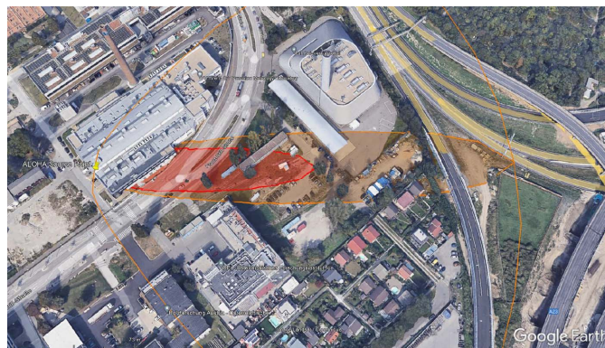
Figure 15: results of the dispersion calculation with heavy gas model for a release of 37 kg SO 2 in 3 min with wind direction west, IDHL zone in red, AEGL-3 zone in orange.
