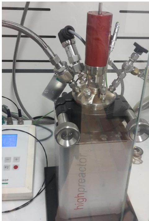
Figure 37 Autoclave used for the hydrothermal synthesis of BZT nanoparticles.
