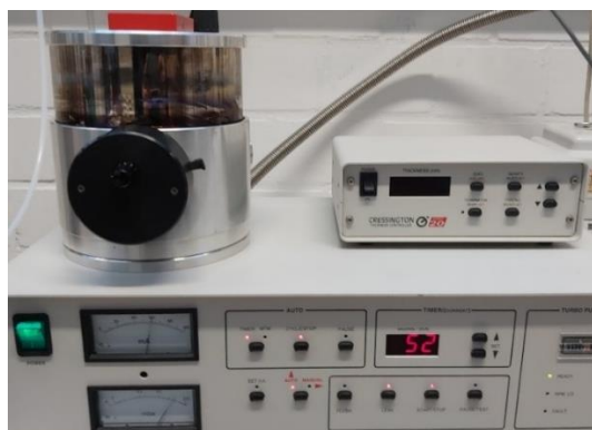
Figure 40 Sputter coater setup for electrode deposition.
