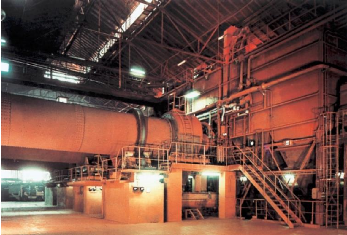
Figure I - 2.1: Rotary kiln in ironoxide pigment production, Lanxess process plant (Krefeld) [6]
