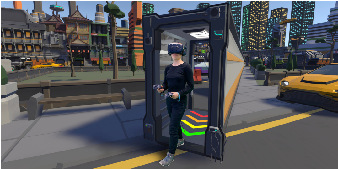
Figure 3.3: Our scaled-walking concept [P4] accelerates the user’s physical steps to traverse larger distances by natural walking. We prevent cybersickness by reducing the visual flow with a virtual tunnel. Windows in the walls provide a peripheral view of the scaled movement.
