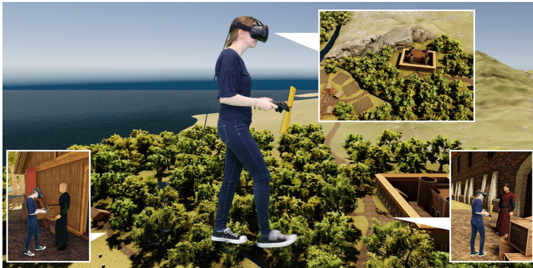
Figure 3.1: With our GulliVR concept [P17], users can transform into a giant on demand and travel large virtual distances by natural walking. Players experience no cybersickness due to the proportional scaling of the eye distance.
