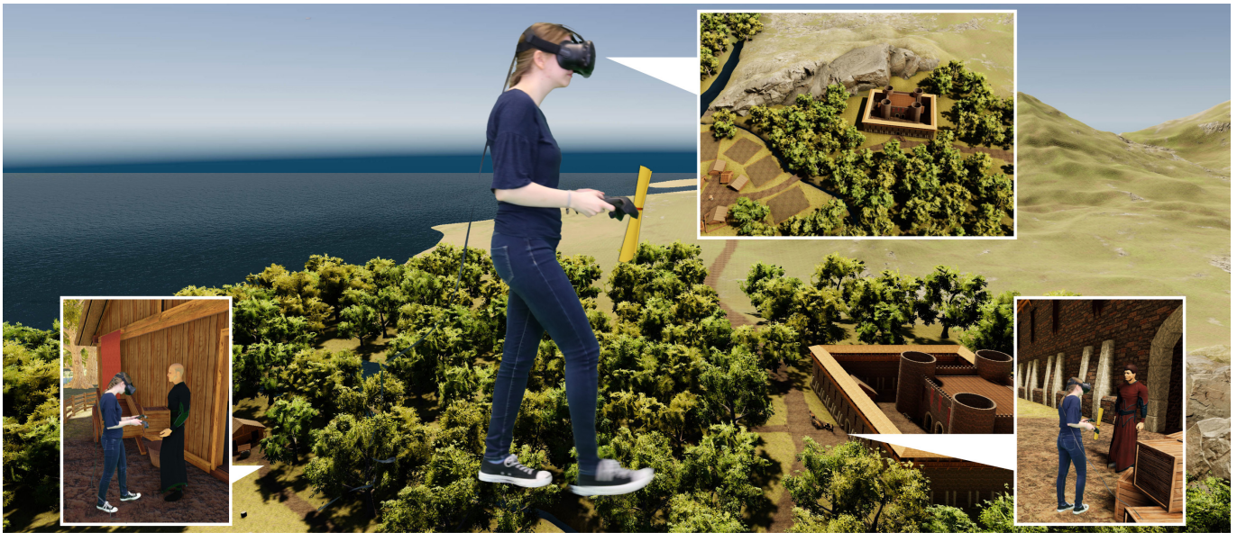
Figure 1. GulliVR allows players to become giants on demand and to traverse larger distances in room-scale VR setups within a few steps. The modeled eye distance is enlarged proportionally to the virtual body size, which ensures the absence of cybersickness.
