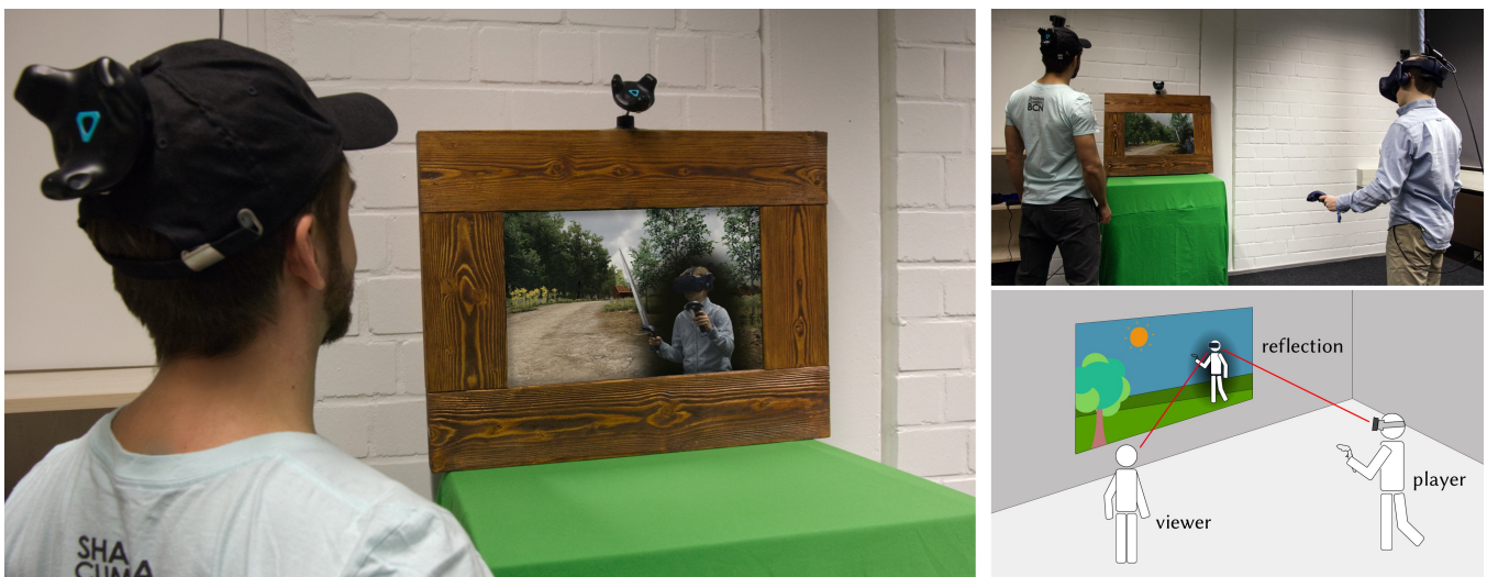
Figure 1: Our paper contributes a new spectatorship experience for virtual reality games. We blend the player’s reflection in the virtual environment and provide a dynamic view frustum that allows viewers to explore the game world by themselves.
