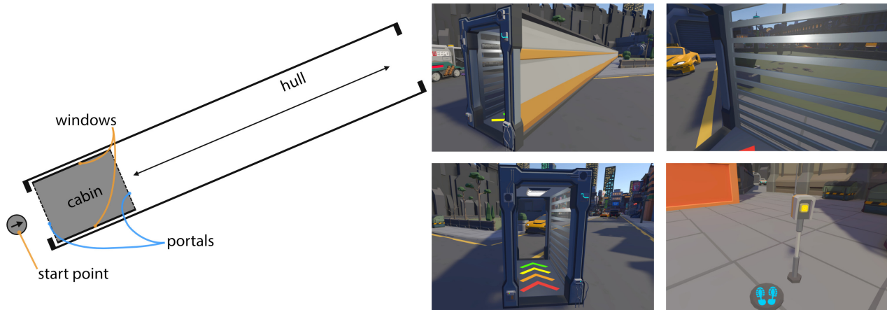
Fig. 2. The virtual tunnel, as the core of our novel locomotion technique: The exterior hull spans from the start point to the target. While users walk through the cabin , it is moved along the tunnel to transport the users to their destination. The cabin’s walls and portals create an optical illusion, whereas the windows provide a view of the accelerated movement. Users initiate the tunnel by standing on a platform and pressing a button.
