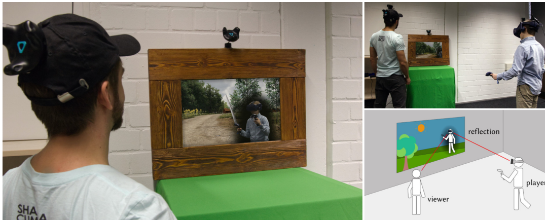
Figure 6.2: Our novel mixed-reality display [P10] allows local bystanders to watch the player's actions in VR by blending the player's real reflection with the virtual surroundings. Observers can change their viewing angle by walking through the play space.
