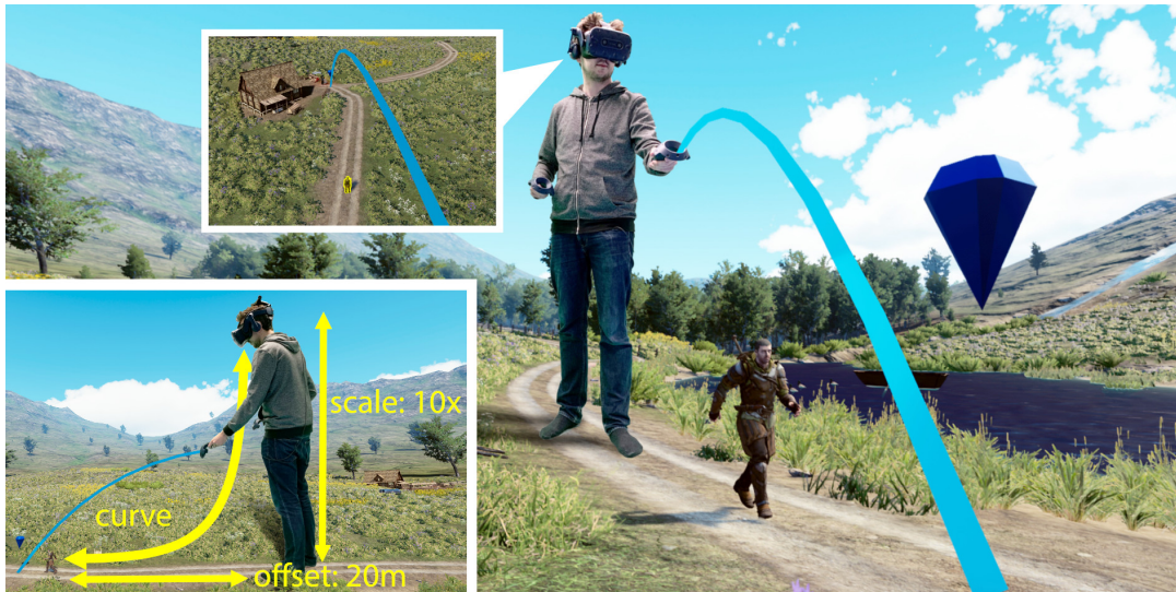
Figure 3.2: Our Outstanding concept [P12] allows users to switch to an enlarged third-person perspective and control their avatar via raycast aiming. Bottom left: We finetuned the transition parameters to convey a feeling of embodying or disembodiment of the avatar.
