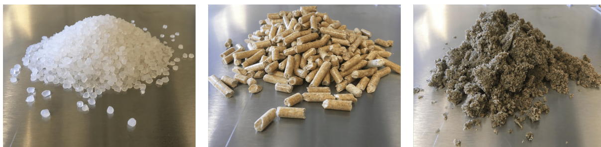
Figure 5.6: Calibrated materials, from left to right: Plastic Granulate; Wood Pellets; Wet Sand [211].
