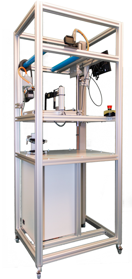
Figure 5.5: Overview of the mobile DEM-Calibration unit [211].
