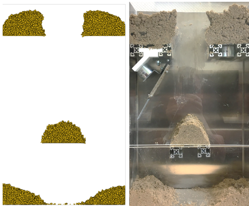
Figure 5.21: Comparison of the validation experiment with wet sand (left: DEM simulation, right: Physical test in calibration unit) [211].
