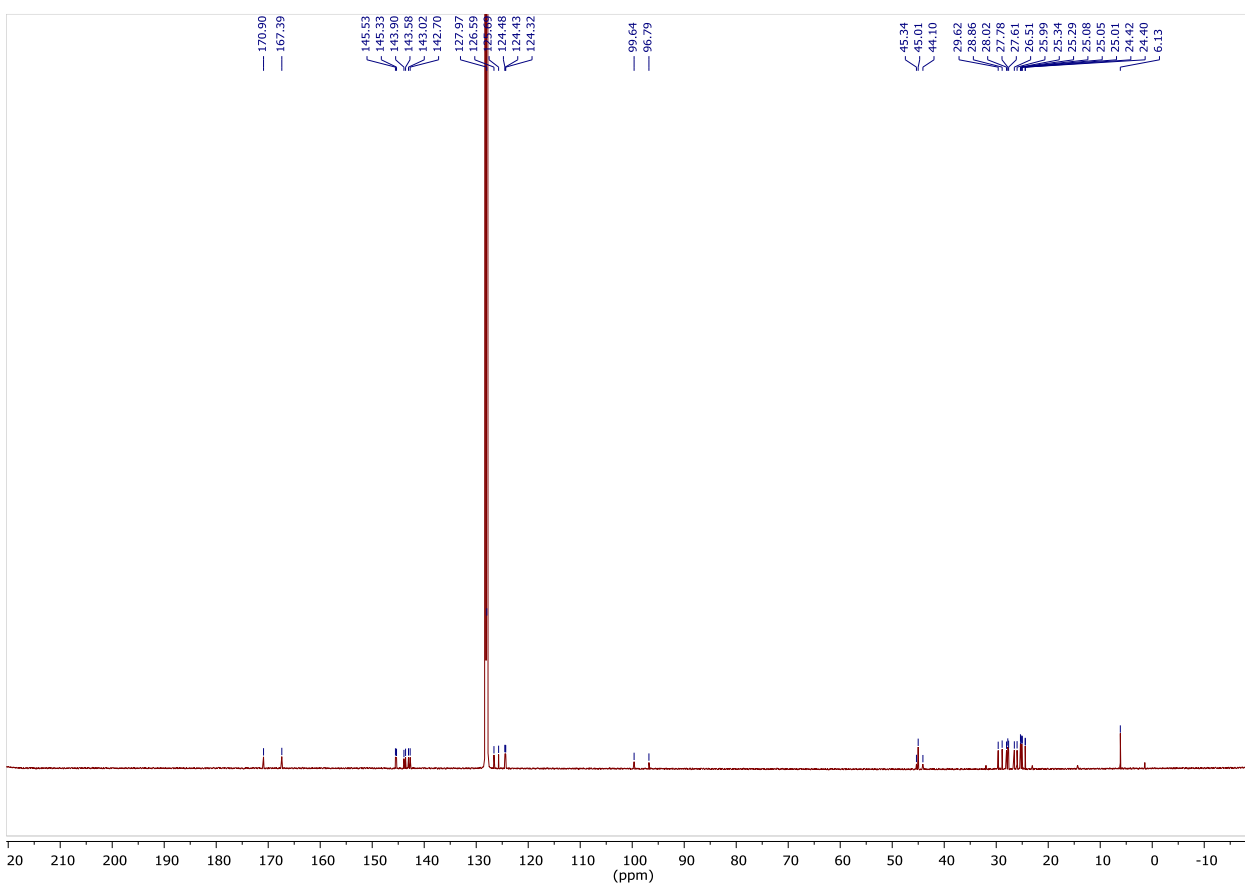
Figure 83: ^{13}\text{C} NMR spectrum (150.9 MHz, \text{C}_6\text{D}_6 , 25 ^\circ\text{C} ) of [\text{L}(\text{Me}_2\text{N})\text{Ga}]\text{SbSb}[\text{N}(\text{SiMe}_3)\text{Ga}(\text{NMe}_2)\text{L}] ( 19 ).
