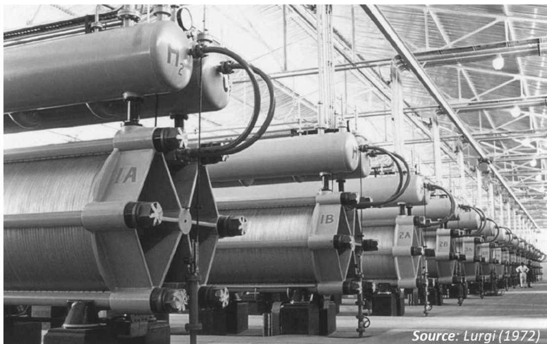
Figure 2-14: Kwe-Kwe Electrolyser Plant for 21,000 Nm 3 /h at 95 MW electrical consumption [48]
