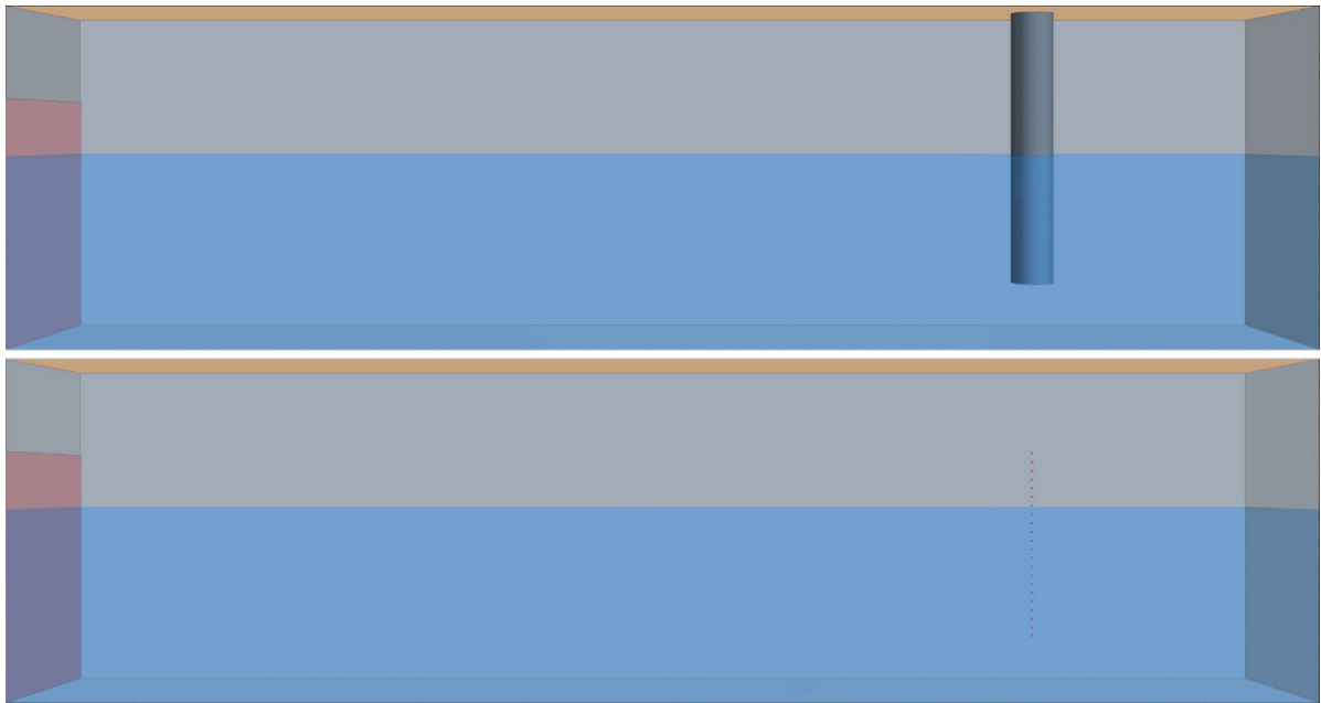
Figure 8. Arrangement of a single cylinder in the first scenario ( top ) and the 210 probe points (only 22 in this figure for illustrative purposes) at which longitudinal velocities were pre-calculated ( bottom ).
