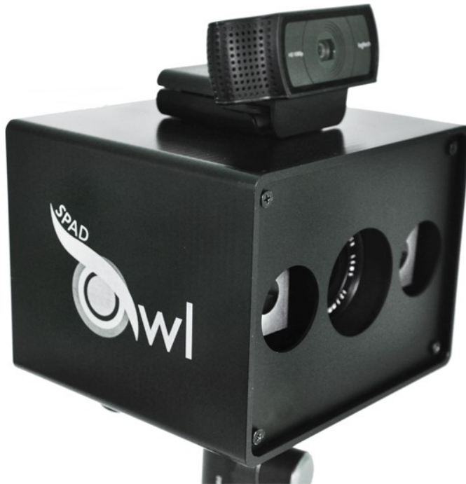
Figure 6.1: Flash LiDAR system “Owl” [101]. On the top is a camera, which is used to capture detection scenes. In the main part of the system, there are two laser sources on the left and right sides and a SPAD detector array in the middle.
