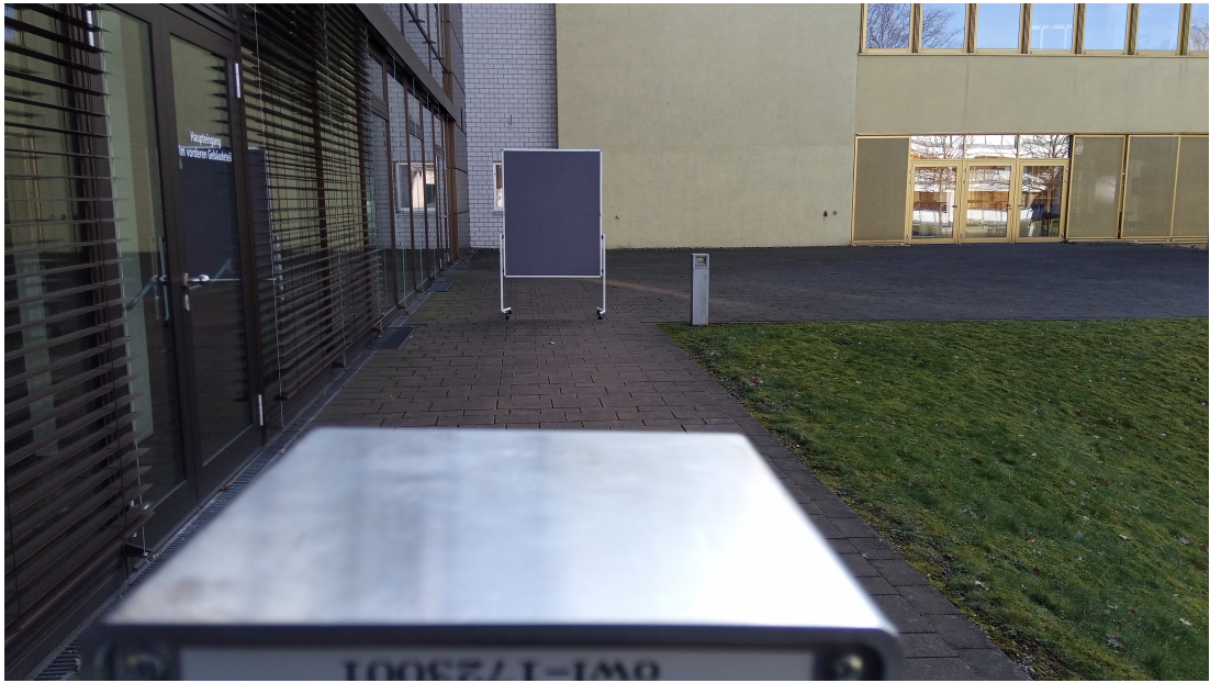
Figure 6.5: Front view of outdoor detection scene. The scene includes an object at 17.50 m, a side wall, and two background walls at 27.50 m and 28 m. r_B is within (1, 3] MHz.
