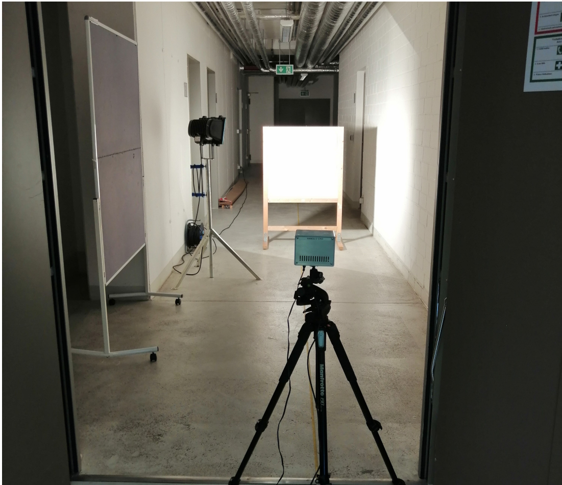
Figure 5.1: Front view of experimental setup. The total length of the basement tunnel is 25 m. A 1.5 m×1.5 m-sized white board is used as the target object. The LiDAR system “Owl” has a two-line SPAD detector array. The lines are positioned 1 degree apart vertically to the ground. Each line is horizontal to the ground and contains 192 pixels. A halogen floodlight is aimed at the object, which creates a maximum r_B of 9 MHz. During the experiment, the object was placed at different distances. The measurement data was accumulated from the 96 th pixel of the upper detector line.
