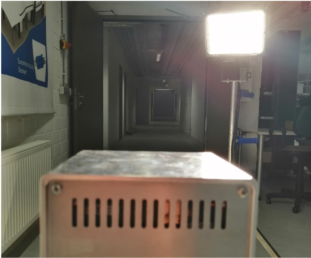
Figure 6.3: Front view of indoor detection scene. The scene includes an object at 20 m, two side walls, and two background walls at 23 m and 27.5 m. A halogen floodlight is aimed directly at the “Owl”. It creates high r_B (from 5 to 10 MHz) over the entire detector array.
